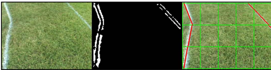
Figure 9: Original image (left), filtered image (middle), classified lines (right).
