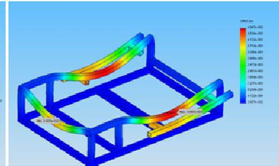
Figure 4: Frame max displacement
