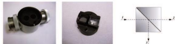
Figure 3. The beam splitter.
