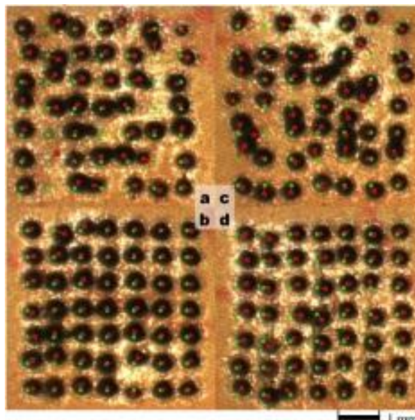
Fig. 15. Results from paper slide trials. Green solid dots indicated preoperatively specified burn locations, and red hollow circles indicate the centroid of the burn. (a) Top left: 0.5 Hz unaided. (b) Bottom left: corresponding aided trial from 0.5 Hz trial. (c) Top right: 1.0 Hz unaided. (d) Bottom right: corresponding aided from 1.0 Hz trial.
